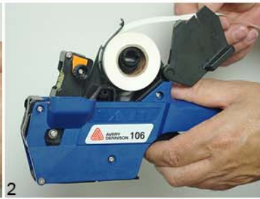
2 Insert roll on label roll holder
