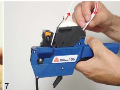
7 Feed the label strip through the body
