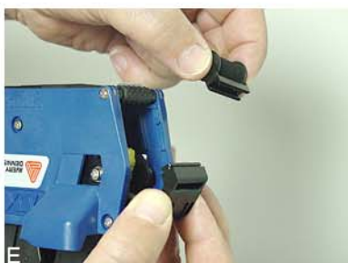
E Slide new ink roller onto the holder & release ink roller holder
