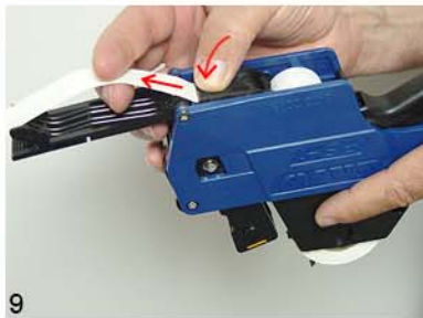
9 To close, press the platen; while pressing, pull label strip until it "clicks" & does not advance
