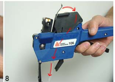
7 Feed the label strip through the body
